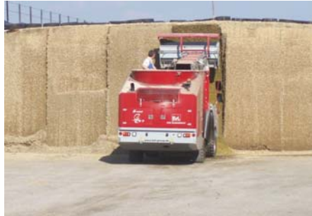
carri miscelatori / self-propelled loading mixers
