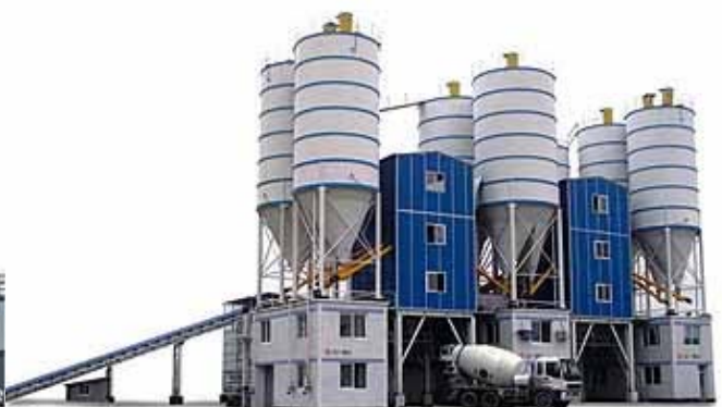
CONCRETE BATCHING PLANT
