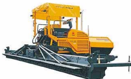
HIGH-GRADE ASPHALT PAVER
